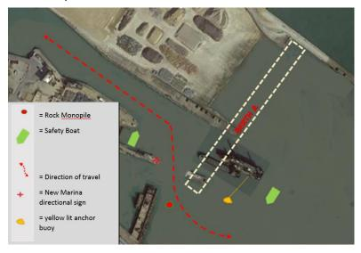
A newly installed red monopile identifies the toeline of the Jet Foil Jetty rock armour to assist vessels to safely navigate through the cut.
